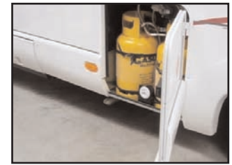
Installation using Mounting Bracket with a 0.6metre hose and right angle adaptor
