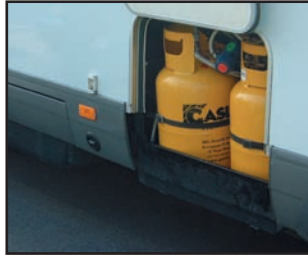
Installation in the skirt below the floor level of a motorhome will require the use of a 1.5metre hose.
