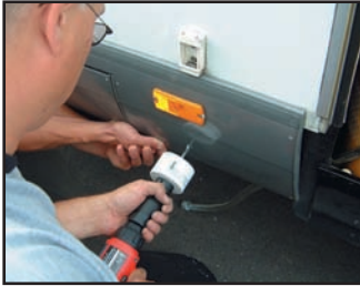
Installation in the skirt below the floor level of a motorhome will require the use of a 1.5metre hose.
