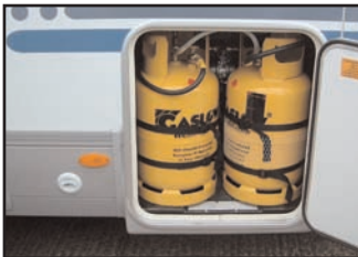
Skirt Installation using a 1.5metre hose.
