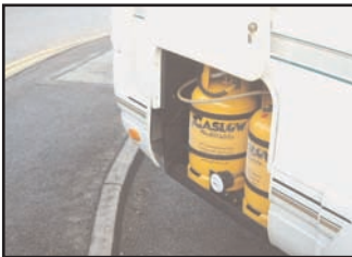
Installation using Mounting Bracket but with a 1.5metre hose and no right angle adaptor
